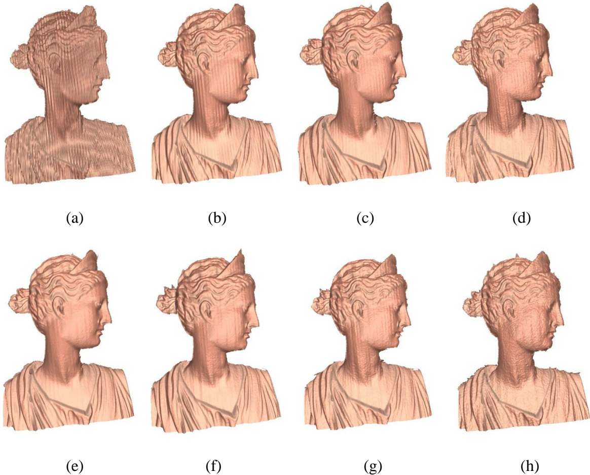
Figure 24. Measurement results of a complex sculpture for the DBP and the FSP methods at different defocusing levels. Level 1 is focused and level 4 is severely defocused. (a)-(d) show the results by the DBP method with defocusing levels from 1 to 4, and (e)-(h) show the results by the FSP method with different levels.
